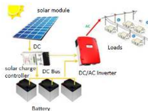
Fig. 3. Scheme or Components PLTS 25 kWp Off Grid on Tunda Island
